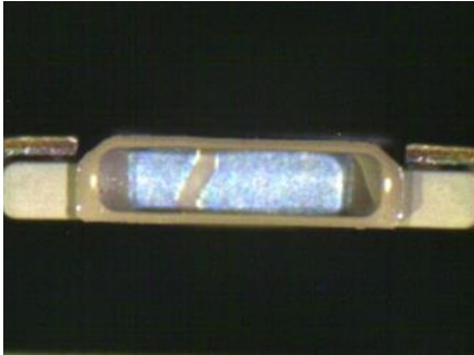
Figure 1. SMD Package After Solder Reflow Testing (aspect ratio 1:4)
