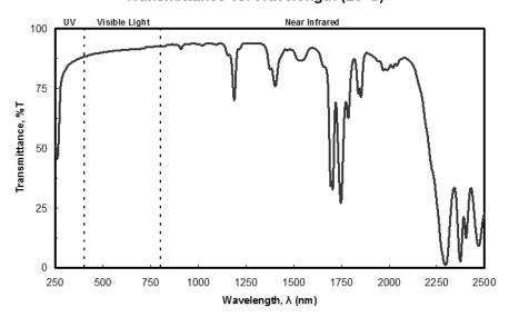
Figure 1. Transmittance spectrum of cured LS1-6140 at a nominal thickness of 0.075" (2 mm)
