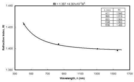
Figure 2. Dispersion curve fit for Refractive Index vs. Wavelength at 25°C
