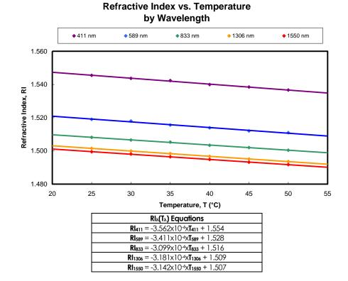
Figure 3. Refractive Index vs. Temperature, at various wavelengths.
